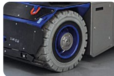
RUOTE ANTISTRACCIA Non-marking tires / Roues non marquant Non-Marking-Räder / Ruedas anti-marcas
