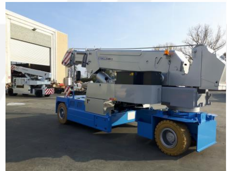
Extendable chassis to increase lifting capacity
