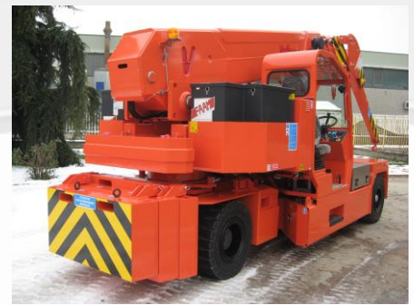
Removable ballasts to make it easier to transport the crane
