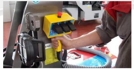
Wired remote control for the aerial part
