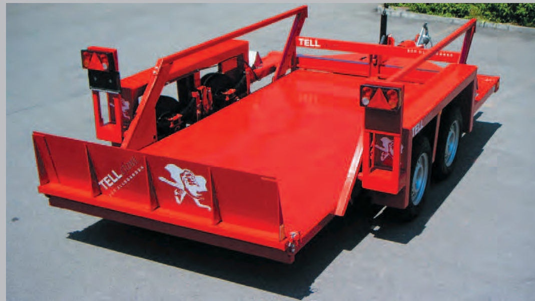
Battery and hydraulic components are integrated with the chassis and are lockable.
