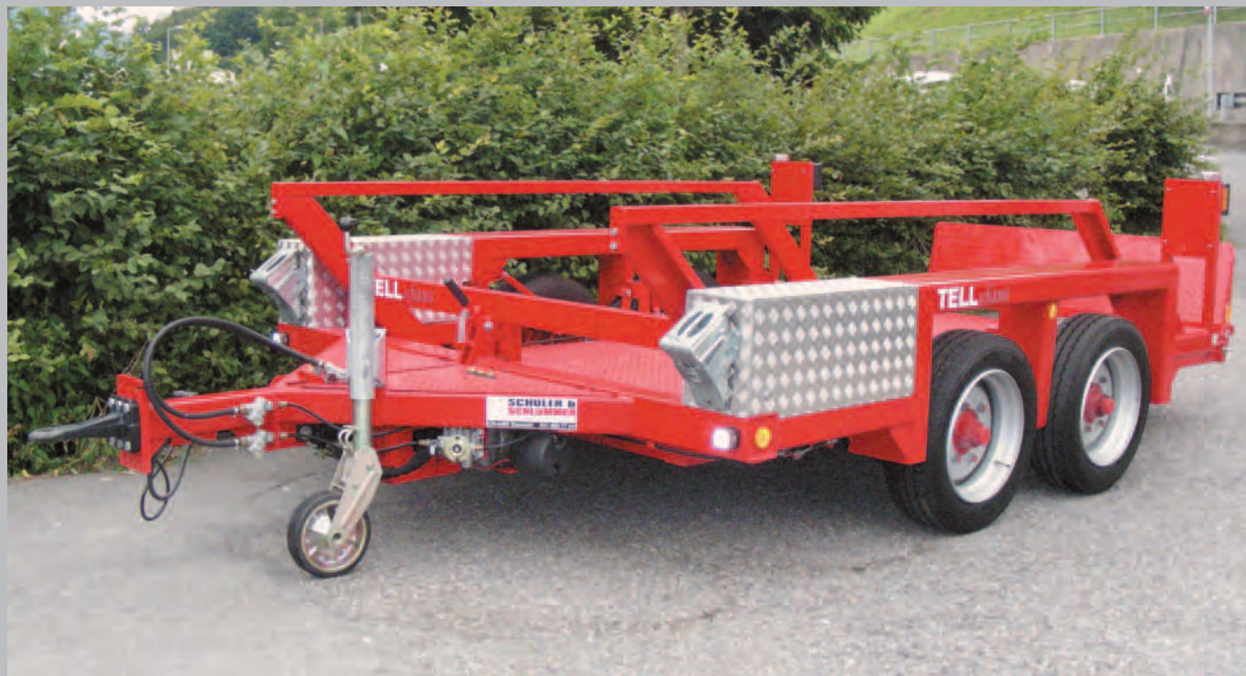
Modified folding ramp provides underride protection
